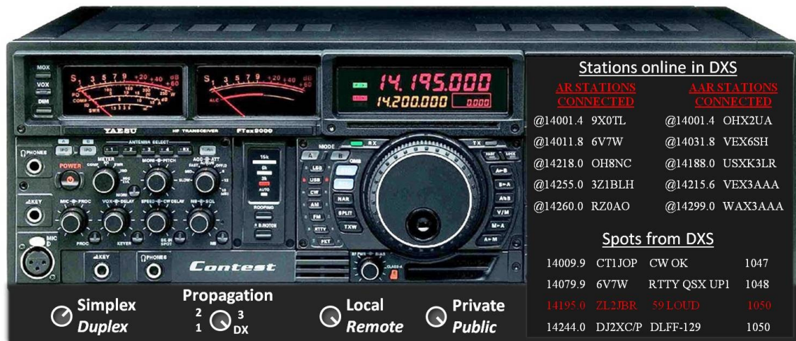
Figure 5: Using the radio's front panel, whether a real radio or a PC screen, you can spin the dial on a virtual or real band but also command a remotely controlled radio. A propagation switch is set to desired band conditions where 1 simulates tough 160m conditions and the DX position opens 20m for solid 48-hour two-way contacts. A simplex / duplex switch is needed since many traditional operators may prefer talking in turns (simplex). A mode switch between public and private may serve the purpose as well.
